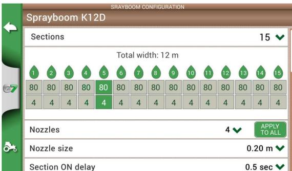
Set-up parameters for boom sprayer
